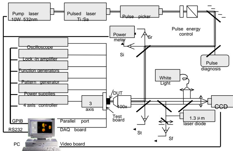
IXL Experimental set-up for ICs testing with a pulsed laser.
