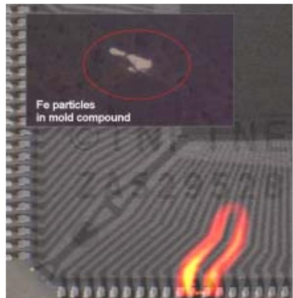
Fig.2: Detail of fig.1. Inset shows metallic grit, visible after mechanical polishing.
