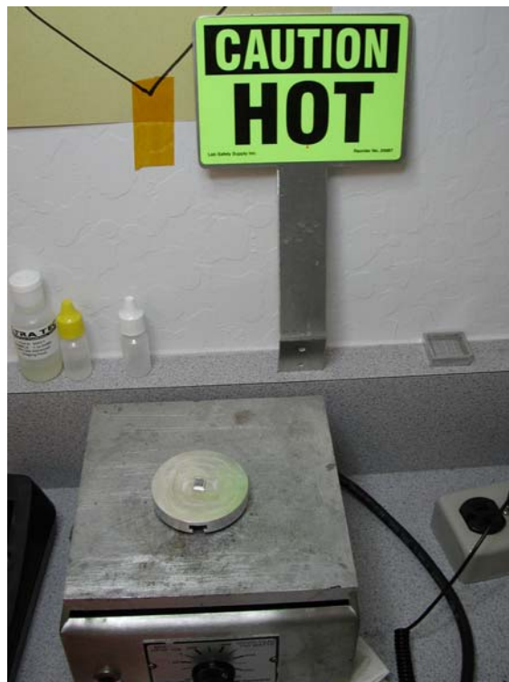
Die being mounted with "crystal bond"
