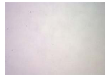
Cloudy surface means not well polished
