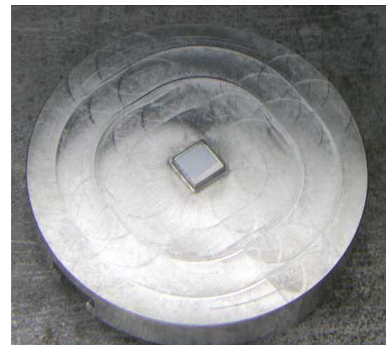
Die thinned & ready to be glued onto support
